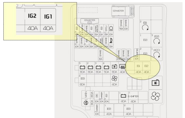
motor compartment fuse box
