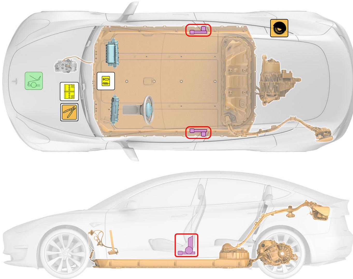
**▲ Warning:** The SRS control unit has a backup power supply with a discharge time of approximately ten seconds. Do not touch the SRS control unit within 10 seconds of an airbag or pre-tensioner deployment.
