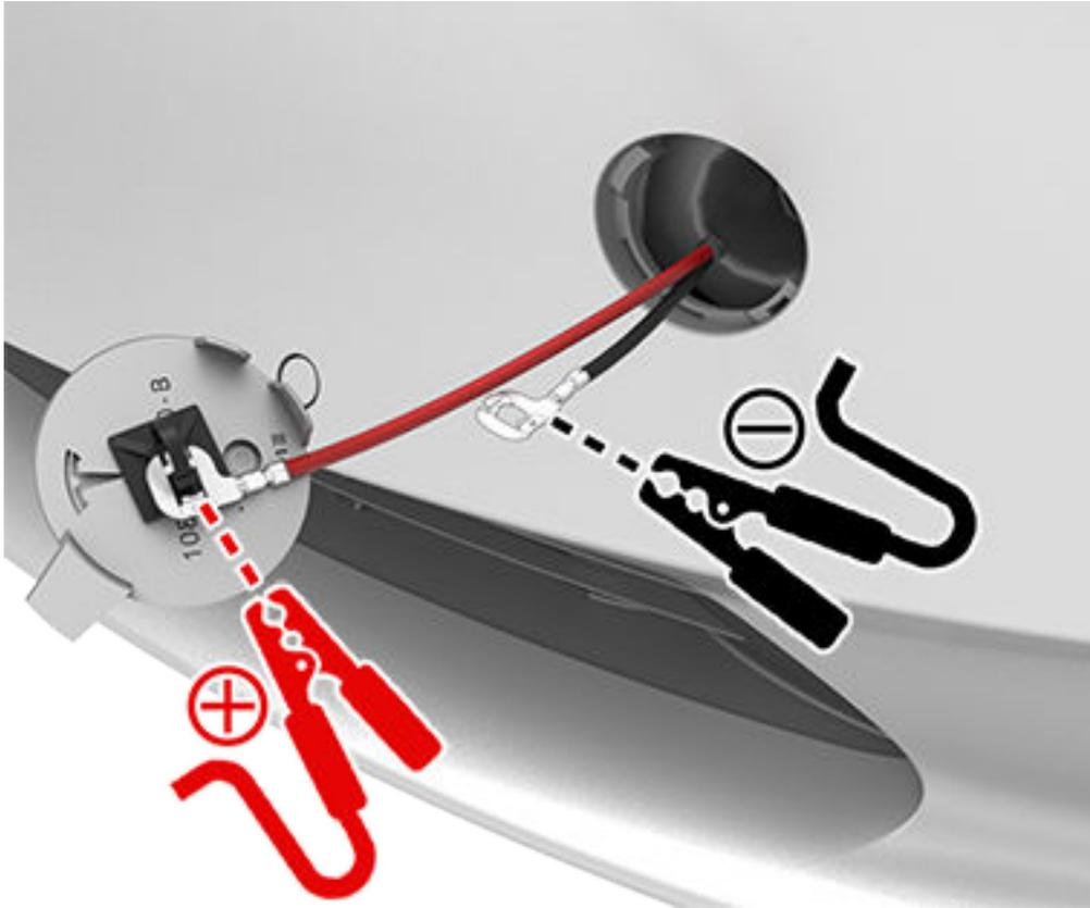
6. Turn on the external power supply (refer to the external power supply manufacturer's instructions). The hood latches are immediately released and you can now open the hood to access the front trunk area.
