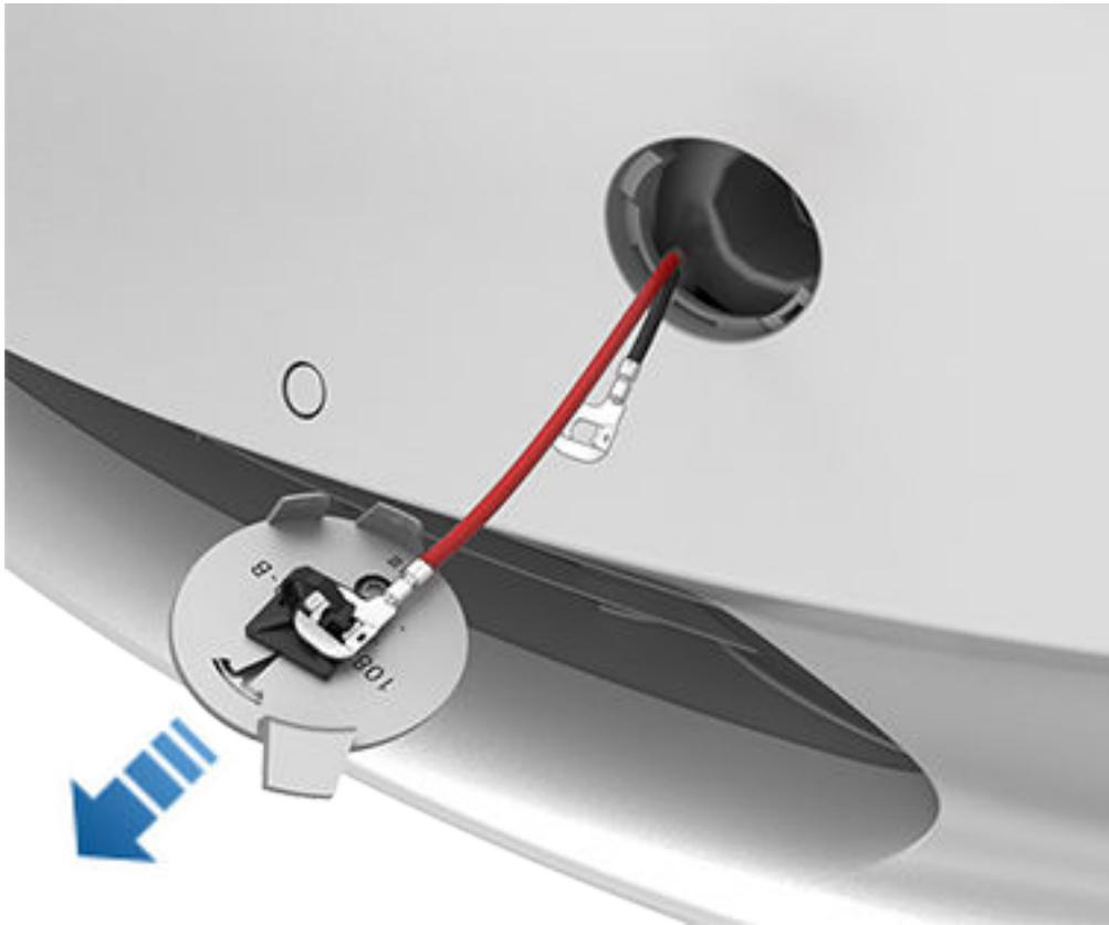
4. Connect the external 12 volt power supply's red positive (+) cable to the red positive (+) vehicle-side terminal.
