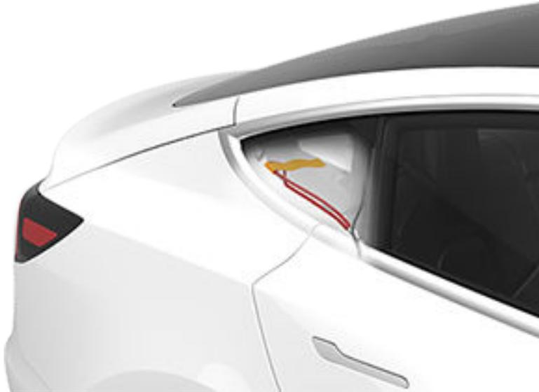
2. Use a reciprocating saw or hydraulic rescue cutters to cut 6 in (15 cm) through the rear pillar in the location shown.
